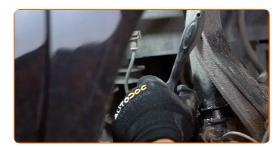
Unscrew the fastening bolt that connects the shock strut with the shock absorber fork. Use a drive socket #14. Use a tap wrench.
