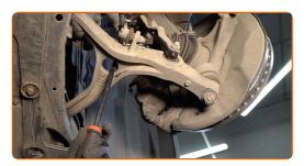
Pull aside the shock strut from its mounting seat.
