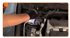
Loosen the upper fastener of the shock strut mount. Use a drive socket #14. Use a ratchet wrench.
