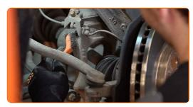
Unscrew the ABS cable holder. Use a drive socket #12. Use a ratchet wrench.
