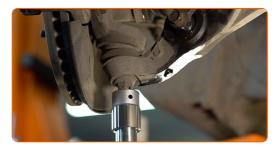
Tighten the fastening bolt that connects the shock strut with the shock absorber fork. Use a drive socket #14. Use a torque wrench. Tighten it to 49 Nm torque.
