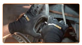
Tighten the ABS cable holder. Use a drive socket #12. Use a ratchet wrench.
