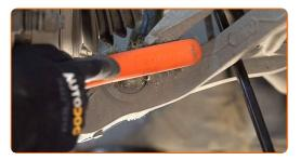
Unscrew the fastening bolt that connects the shock absorber fork with the lower control arm. Use a combination spanner #17. Use a drive socket #17. Use a tap wrench.
