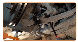
Detach the shock absorber fork from the shock strut. Use a flat metal-working chisel. Use a hammer.
