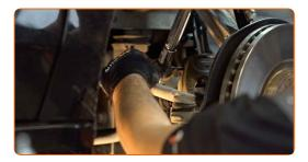
Tighten the fastening bolt that connects the shock absorber fork to the lower control arm. Use a combination spanner #17. Use a drive socket #17. Use a torque wrench. Tighten it to 64 Nm torque.
