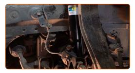
Remove the support from under the arm.
