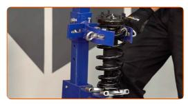
Remove the assembled shock strut.
