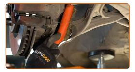
Attach the shock absorber fork to the shock strut.
