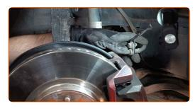
Remove the suspension strut.
