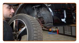
Clean the shock strut fasteners. Use a wire brush. Use WD-40 spray.
