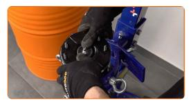
Tighten the shock strut piston rod nut. Use a combination spanner #17. Use HEX No.H6. Use a torque wrench. 33 Tighten it to 29 Nm torque.
