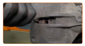
Remove the brake caliper. Use a crowbar.
