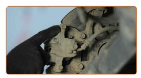
Unscrew the brake caliper fastening. Use a combination spanner #17. Use a drive socket #12. Use a ratchet wrench.
