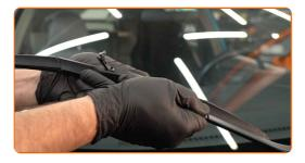
Remove the blade from the wiper arm.
