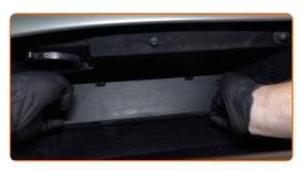
Remove the cabin air filter housing.
