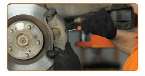
10 Remove the brake caliper.
