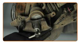
19.1 Install the brake caliper and fix it.
