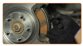
Remove the brake pads. Use a crowbar.
