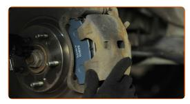
19.2 Use a drive socket #12. Use a torque wrench. Tighten it to 34 Nm torque.
