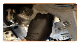
Screw in the new drainage plug and tighten it. Use a drive socket #17. Use a torque wrench. Tighten it to 39 nm torque.
