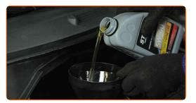
Replacement: engine oil and filter – HONDA Accord VI Coupe (CG). Tip:
