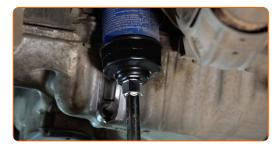
Prepare a container for the old oil filter. Put the old oil filter in the container.
