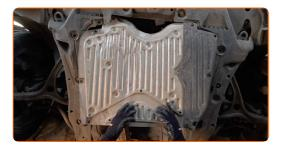
Screw in the fasteners of the lower sound insulation. Use a drive socket #10. Use a ratchet wrench.
