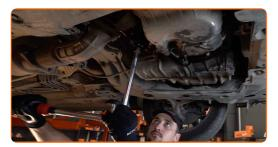
Replacement: engine oil and filter – HONDA Accord I Hatchback (SJ, SY). AUTODOC recommends:
