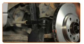
17 Tighten the fastening nut connecting the tie rod end to the steering knuckle. Use a drive socket #18. Use a torque wrench. Tighten it to 30 Nm torque.+90°
