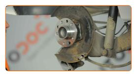
Tighten the wheel hub bolts. Use a drive socket #16. Use a torque wrench. Tighten it to 50 Nm torque.+45°
