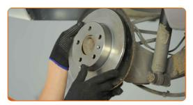
Unscrew the wheel hub bolts. Use a drive socket #16. Use a ratchet wrench.
