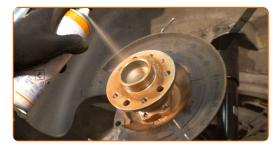
22 Install the brake disc.
