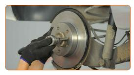
12 Remove the brake disc.
