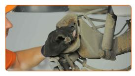
Remove the brake disc cover.
