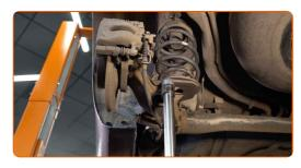
Unscrew the lower fastener of the shock absorber. Use a drive socket #E20. Use a ratchet wrench.
