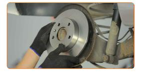
Tighten the brake disc fastening. Use Torx T30. Use a torque wrench. Tighten it to 4 Nm torque.
