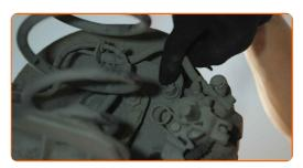
Unscrew the caliper bracket fastening. Use a drive socket #E18. Use a ratchet wrench.
