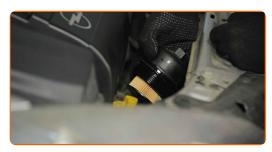
Use a drive socket #27. Use a torque wrench. Tighten it to 25 Nm torque.
