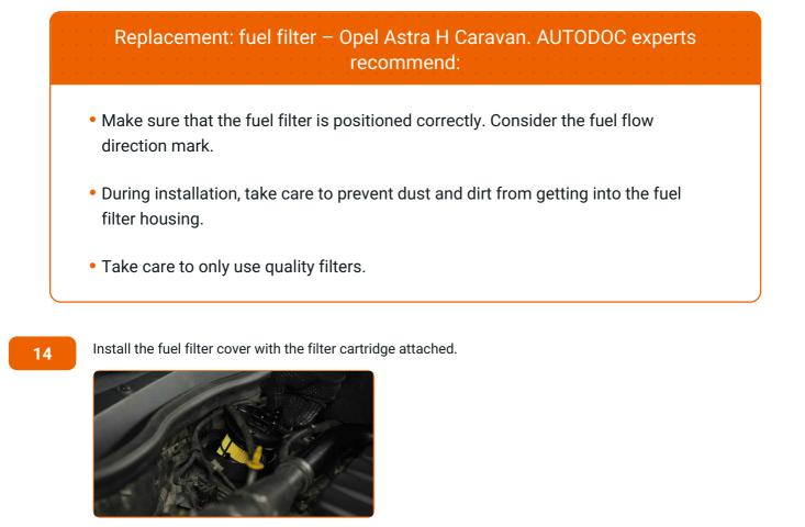
Tighten the fasteners of the fuel filter housing cover.
