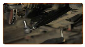
Connect the ball joint to the steering knuckle. Use a rubber mallet.
