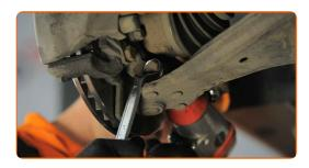
Remove the fastening bolt.
