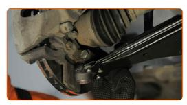
Tighten the fastener connecting the ball joint to the steering knuckle. Use a combination spanner #18. Use a drive socket #18. Use a torque wrench. Tighten it to 50 Nm torque.
