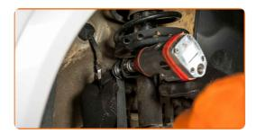
Tighten the fastener connecting the stabilizer link to the stabilizer bar. Use a combination spanner #18. Use Torx T30. Use a torque wrench. Tighten it to 60 Nm torque.
