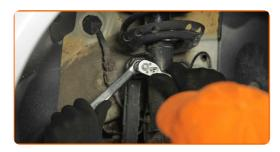
Unscrew the fastener connecting the stabilizer link to the stabilizer bar. Use a combination spanner #18. Use Torx T30. Use a ratchet wrench.
