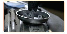
Take out the ignition coils from the spark plug wells.
