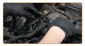
Connect the ground wires to the ignition coils and screw in the fasteners. Use a drive socket #10. Use a ratchet wrench.
