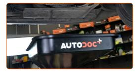
Clean the area of the oil pan drainage hole. Use a nylon cleaning brush. Use all-purpose cleaning spray.
