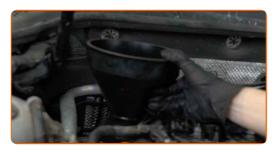
Pour oil into the engine through the filler. Required amount of oil: 4.7 l.
