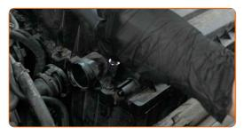
Connect the vacuum hose to the air filter housing.
