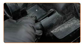
Connect the crankcase breather hose to the air filter housing.
