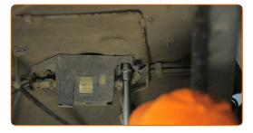
Remove the fuel filter together with its bracket.
