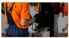
Unscrew the fuel filter bracket fixing bolts. Use a drive socket #17. Use a ratchet wrench.
