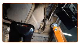
Loosen the fuel supply lines fastening to the fuel filter. Use a flat screwdriver.
