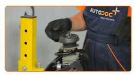
Tighten the shock strut piston rod nut. Use a drive socket #21. Use a torque wrench. Tighten it to 65 Nm torque.
