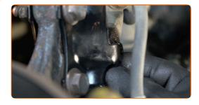
Tighten the brake hose fastening bracket to the shock strut. Use a drive socket #10. Use a ratchet wrench.
