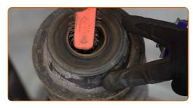
Remove the strut piston rod nut. Use a drive socket #21. Use a ratchet wrench.
