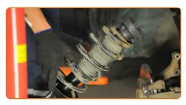
Set the shock absorber strut on the spring compressor tool.
