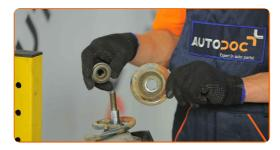
Release the coil spring.
