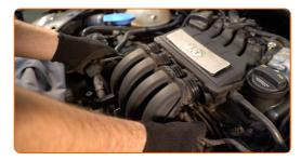
Tighten the intake manifold fasteners. Use a Phillips screwdriver.
