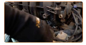
Detach the retainers of the ignition cables.
