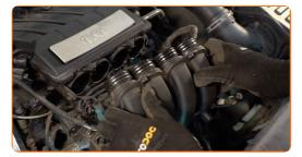
Cover the intake manifold passages with a microfibre towel to prevent dust and dirt from getting inside.
