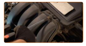
11 Remove the intake manifold.
