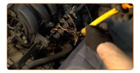
Unscrew the intake manifold fasteners. Use HEX No.H6. Use a drive socket #13. Use a ratchet wrench.
