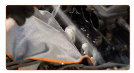
Treat the spark plug wire connectors. Use high-temperature grease. Use a flat screwdriver.
