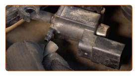
Unscrew the intake manifold fasteners. Use a Phillips screwdriver.
