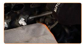
Screw new spark plugs and tighten them. Use the spark plug socket #16. Use a torque wrench. Tighten it to 25 nm torque.
