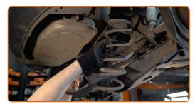
Install the coil spring together with the rubber mounts into the mounting seats. Use a crowbar.
