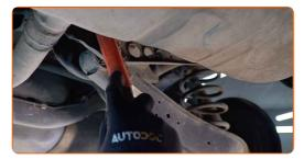
Make a mark on the camber adjustment bolt.
