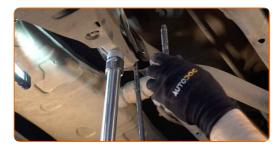
11 Remove the support from under the arm.
