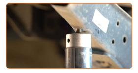
Remove the fastening bolt. Use a crowbar.
