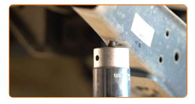
Remove the fastening bolt. Use a crowbar.
