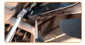
Remove the support from under the arm.
