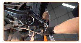
Screw in the fasteners connecting the control arm to the rear knuckle. Use a combination spanner #18. Use a drive socket #18.
