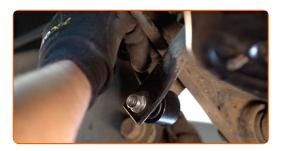
Tighten the fastener connecting the stabilizer link to the stabilizer bar. Use a combination spanner #14. Use XZN #6. Use a drive socket #15. Use a torque wrench. Tighten it to 45 Nm torque.
