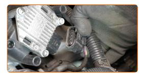
Unscrew the ignition coil bolts. Use HEX No.H5. Use a ratchet wrench.
