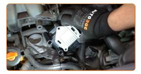
Tighten the ignition coil bolts. Use HEX No.H5. Use a torque wrench. Tighten it to 7 nm torque.
