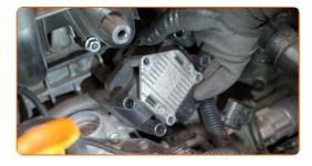
Install the new ignition coil to the spark plug well.
