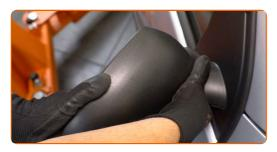
Carefully release the mirror glass from its attachment. Use a plastic trim tool.
