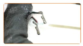
6 Attach the mirror heating connectors.
