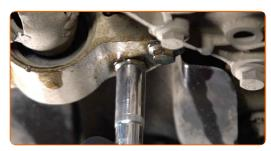
Remove the fastening bolts. Use a drive socket #18. Use a drive socket #16.
