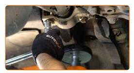
Unscrew the rear fastener connecting the control arm to the subframe. Use a drive socket #16. Use a tap wrench.
