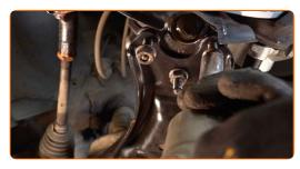
Install the rear fastener of the arm.
