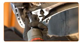
Loosen the front fastener of the control arm. Use a drive socket #18. Use a tap wrench.
