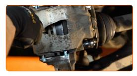
14 Remove the brake caliper.
