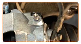
Remove the brake hose clamp.
