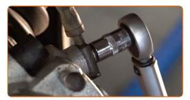
20 Undo the brake bleeder screw. Use a combination spanner #10.
