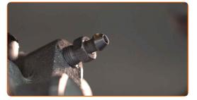
Tighten the brake caliper bleed screw. Use a drive socket #10. Use a torque wrench. Tighten it to 10 Nm torque.
