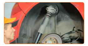
Remove the protective cap of the shock absorber mount. Use a flat screwdriver.
