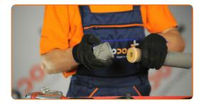
Install the new mount, boot, and bump stop on the shock absorber.
