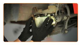
Use HEX No.H7. Use a torque wrench. Tighten it to 30 Nm torque.
