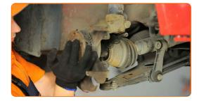
Connect the lower arm to the steering knuckle. Use a crowbar.
