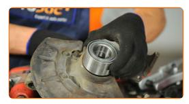
Install the retaining ring. Use circlip pliers.
