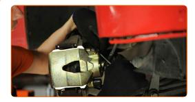
7.1 Unscrew the brake caliper fastening.
