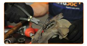
Press out the wheel hub bearing.
