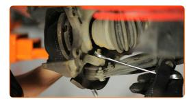
Disconnect the lower arm from the steering knuckle. Use a hammer. Use a crowbar.
