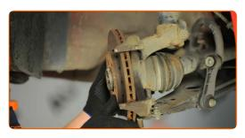
41.1 Install the brake caliper and fix it.
