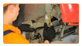
Tighten the lower fastening of the shock absorber. Use a combination spanner #18. Use a drive socket #18. Use a torque wrench. Tighten it to 60 Nm torque.+90°
