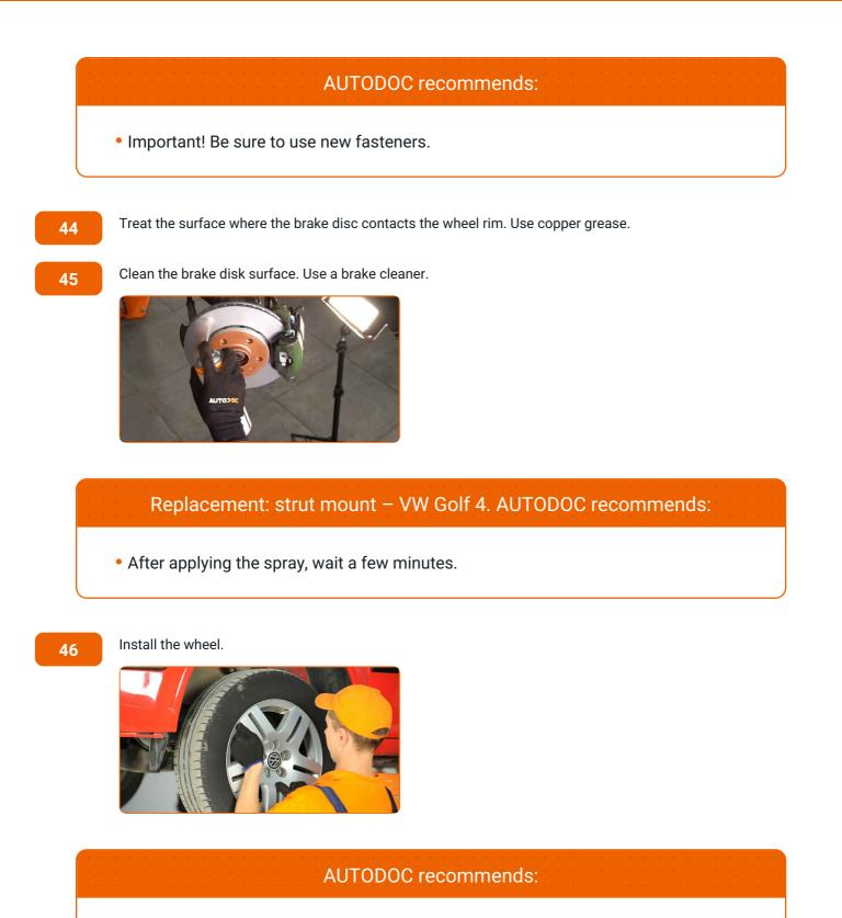
• Important! Hold the wheel while screwing in the fastening bolts. VW Golf 4
