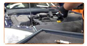
Apply a thin layer of a special high temperature anti-seize lubricant to the threads of the new spark plugs.
