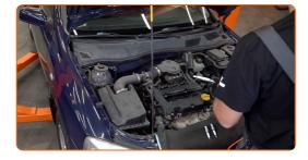
Screw new spark plugs and tighten them. Use the spark plug socket #16. Use a torque wrench. Tighten it to 24 nm torque.
