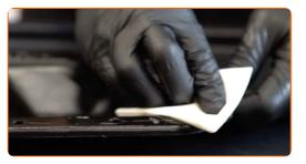
Apply sealant to the mounting seat of the transmission fluid pan gasket. Install the new transmission fluid pan gasket.
