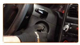
Pull the windscreen wiper stalk to the downward position. By doing so, you will switch the windscreen wipers from the service mode to the operation mode.
