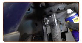
Unscrew the nut and remove the stabilizer rod from the shock strut. Use a combination spanner #19. Use a drive socket #18.
