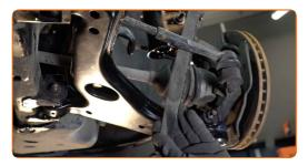
11.1 Install a new rod, tighten the fasteners.
