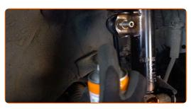
Clean the wheel rim mounting seat. Use a wire brush. Treat the contacting surface. Use copper grease.
