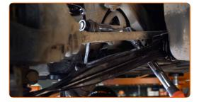
Use a combination spanner #19. Use a drive socket #18. Use a torque wrench. Tighten it to 65 Nm torque.
