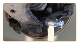
Unscrew the front arm fastener. Use a drive socket #18. Use a combination spanner #18. Use a ratchet wrench.
