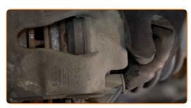
9 Unscrew the brake caliper fastening. Use HEX No.H7. Use a ratchet wrench.
