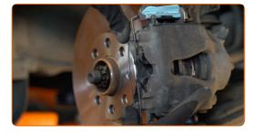
Fasten the brake hose on the strut.
