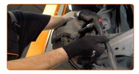
Remove the fastener attaching the brake hose to the shock strut. Use a crowbar.
