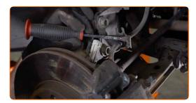
Pull aside the brake caliper retaining spring. Use a crowbar.
