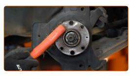
17 Install the brake disc.
