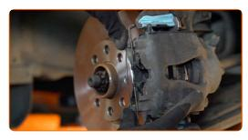
Fasten the brake hose on the strut.
