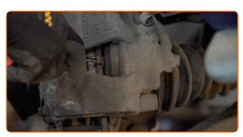
Remove the dust boot caps of the brake caliper guide pins. Use a flat screwdriver.
