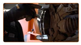
Install the brake caliper and fix it.
