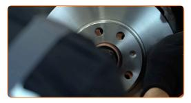
Tighten the brake disc fastening. Use Torx T30. Use a torque wrench. Tighten it to 7 Nm torque.
