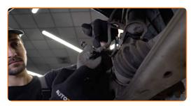
25 Snap the brake caliper retaining spring back into place.
