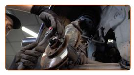
15 Remove the brake disc.
