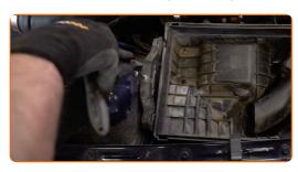
9 Remove the air filter housing.
