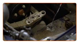
23 Install the engine mount to its mounting seat.
