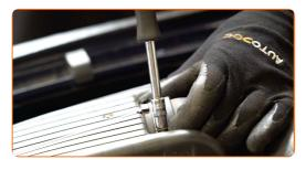
Remove the fender protection cover.
