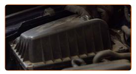
Attach the fasteners connecting the air pipe and the wiring harness to the air filter housing.
