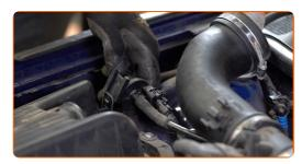
Take off the filter lid. Remove the filter element from the filter housing.
