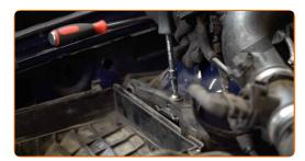
Insert the filter cartridge into the filter housing. Make sure that the filter edge fits tight to the housing.
