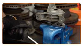
Unscrew the engine mount from the bracket. Use Torx T55. Use a ratchet wrench.
