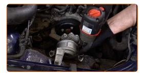
Remove the support from under the engine.
