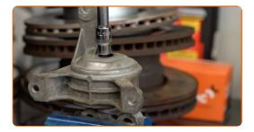
Screw the new engine mount to the bracket. Use Torx T55. Use a ratchet wrench.
