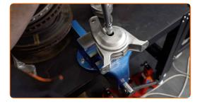
Remove the bracket with the engine mount from the vice.
