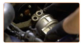
Screw in the engine mount fasteners (6 pieces). Use a drive socket #E20. Use a torque wrench. Tighten it to 55 Nm torque.
