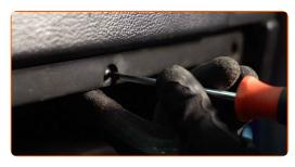
Remove the fender protection cover.
