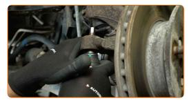
Having adjusted the tie rod end to the correct position, secure it with the lock nut.
