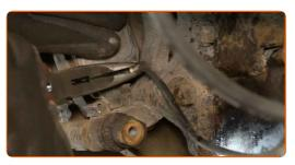
Remove the brake pads.
