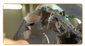
Replacement: brake caliper bracket – FORD Transit V363 Platform / Chassis (FED, FFD). AUTODOC recommends:
