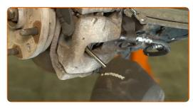
Unscrew the brake caliper fasteners. Use a 13 mm combination spanner.
