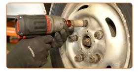
Lower the car and tighten the wheel nuts in a criss-cross order. Use a 21 mm wheel impact socket. Use a torque wrench. Tightening torque: 200 N·m.
