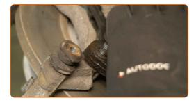
Remove the brake caliper bracket.
