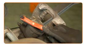
Retract the brake caliper piston. Use a brake caliper wind back tool.
