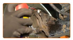
Unscrew the brake caliper bracket fasteners. Use an 15 mm combination spanner.
