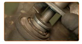
Install a new brake caliper bracket.
