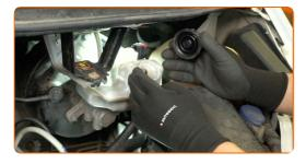
Tighten the brake fluid reservoir cap.
