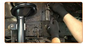
Treat the ABS sensor connector. Use an electronic spray.
