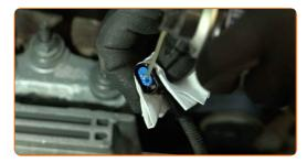
Attach the ABS sensor connector.
