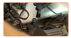
Detach the ABS sensor wiring. Use a plastic trim removal tool. Use a clip removal tool.
