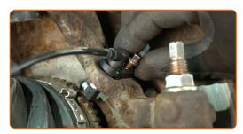
Tighten the ABS sensor fastener. Use an 8 mm socket. Use a torque wrench. Tightening torque: 11 N·m.
