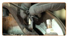
Clean the mounting seat of the ABS sensor. Use a wire brush. Use an all-purpose cleaning spray.
