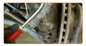
Measure and note down the length of the exposed portion of the tie rod thread or the number of turns the tie rod end made when being unscrewed to prevent wheel misalignment during reassembly. Use a vernier caliper.
