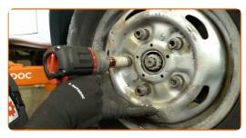
Lower the car and tighten the wheel nuts in a criss-cross pattern. Use a 21 mm wheel impact socket. Use a torque wrench. Tightening torque: 200 N·m.
