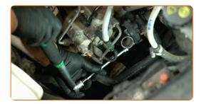
Remove the towel from the coolant hose and reattach it. Use hose clamp pliers.
