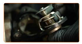
Clean the mounting seat of the thermostat housing cover. Use an all-purpose cleaning spray.
