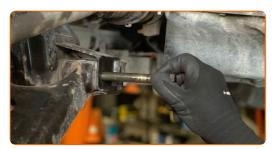
Remove the control arm. Use a mounting lever.
