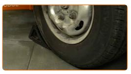
Loosen the wheel nuts. Use a 21 mm wheel impact socket. Use a tommy bar.
