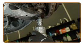
Jack up the steering knuckle. Use a transmission jack or an additional vehicle jack.
