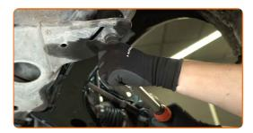
To tighten the fasteners correctly, you have to jack up the suspension to load it. Use a transmission jack or an additional vehicle jack.
