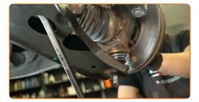
Tighten the fastener that connects the control arm to the ball joint. Use a 24 mm socket. Use a torque wrench. Tightening torque: 150 N·m.
