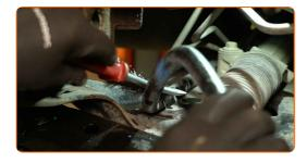
18 Install a new anti-roll bar bush on one side of the axle.
