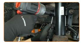
Remove the anti-roll bar link.
