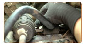
Remove the anti-roll bar bush bracket.
