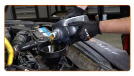
Replacement: engine oil and filter – FORD TRANSIT Platform/Chassis (T\_ \_). Professionals recommend:
